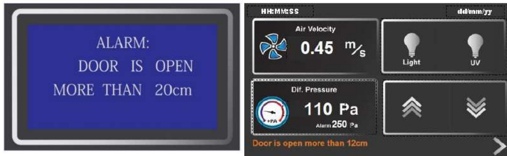
Figure 4-5. Sash opening more than limit
