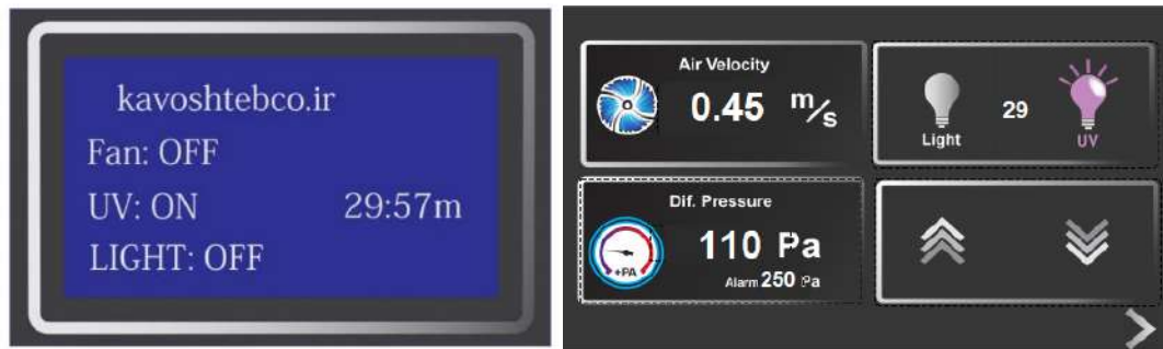
Figure 4-7. UV disinfection cycle
